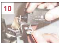
10 With switch positioned and held in place as fig. 9 remove backing from adhesive tape, press sub plate firmly up to bracket with 2 screws protruding through
