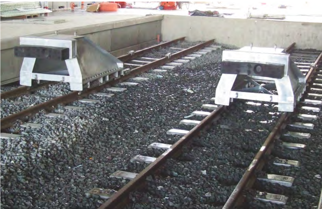
Train mass: 450 tonnes Impacting speed 15km/h fitted with eight pairs of friction shoes with an installation length of 15m.
