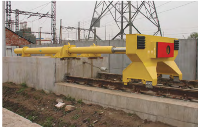
Typically used on metro and main lines – designed for centre and side impact. Concrete base foundation incorporating Oleo hydraulic units (two Oleo Type 724 – Recoverable stroke 2400mm). Train mass: 300 tonnes, Impacting speed: 14km/h, Installation length: 8 metres, Impact capacity 2688kj.
