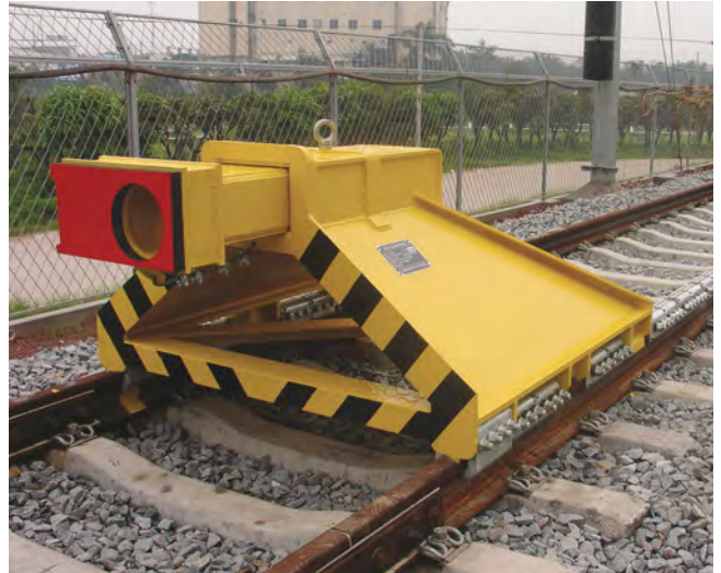
Typically used on metro lines – designed for centre impact only. Sliding friction end stop (twenty friction shoes) incorporating Oleo hydraulic unit (single Type 9 – Recoverable stroke 400 mm). Train mass: 220 tonnes. Impacting speed: 25 km/h. Installation length: 16 metres. Impact capacity: 224kj.
