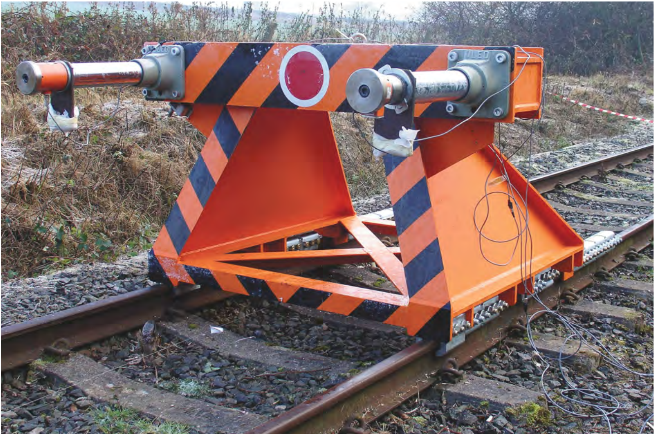
Typically used on European main lines (freight) – designed for side impact only. Sliding friction end stop (eight friction shoes) incorporating Oleo hydraulic units (two Oleo Type 9 – Recoverable stroke 400mm). Train mass: 220 tonnes, Impacting speed: 25 km/h, Installation length: 25 metres, Impact capacity: 448kj.
