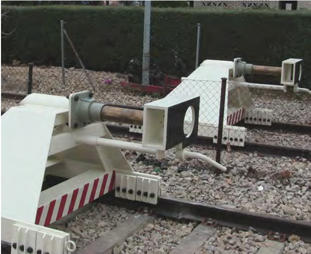
Used on Metro Madrid Series Trains 5000, 6000, 7000, 8000 and 9000. Incorporating Oleo hydraulic unit (one Type 9 – Recoverable stroke 400mm). Train mass range between 163 tonnes and 216 tonnes. Impacting speed maximum 15km/h. Installation length: 7.1 metres. Impact capacity 224kj.
