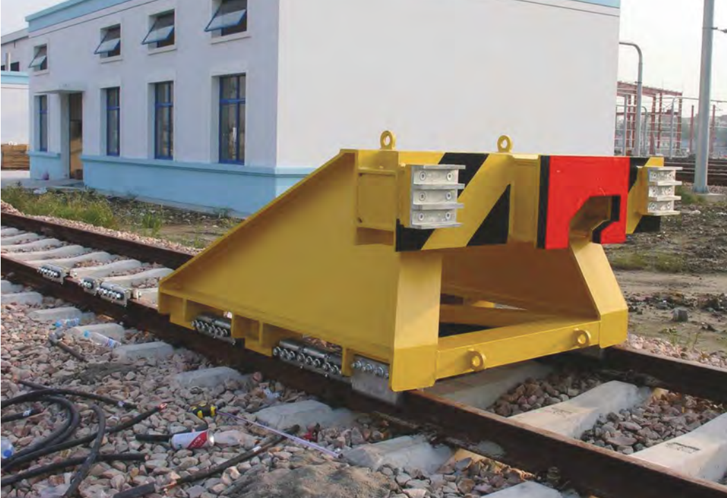
Train mass: 408 tonnes Impacting speed 25km/h fitted with seventeen pairs of friction shoes with an installation length of 15m. Train mass: 252 tonnes Impacting speed 15km/h fitted with eleven pairs of friction shoes in an installation length of 15m.
