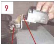
Lever lightly touching push rod
